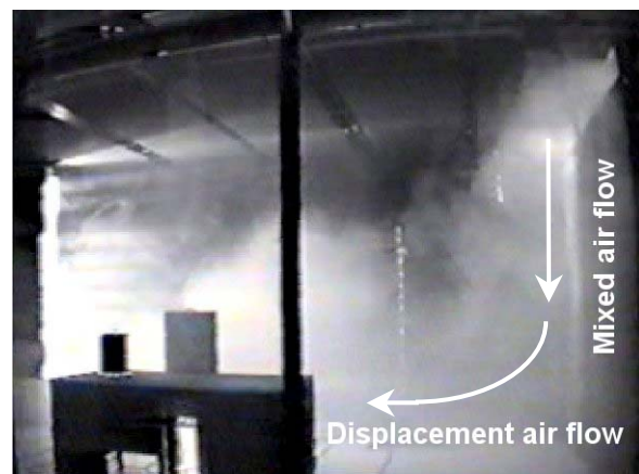
Mixed/displacement air flow principle
