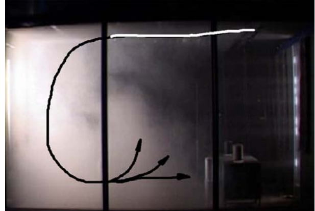
Room air flow technology. Visualization possible in the LTG lab (LTG Engineering Services)
